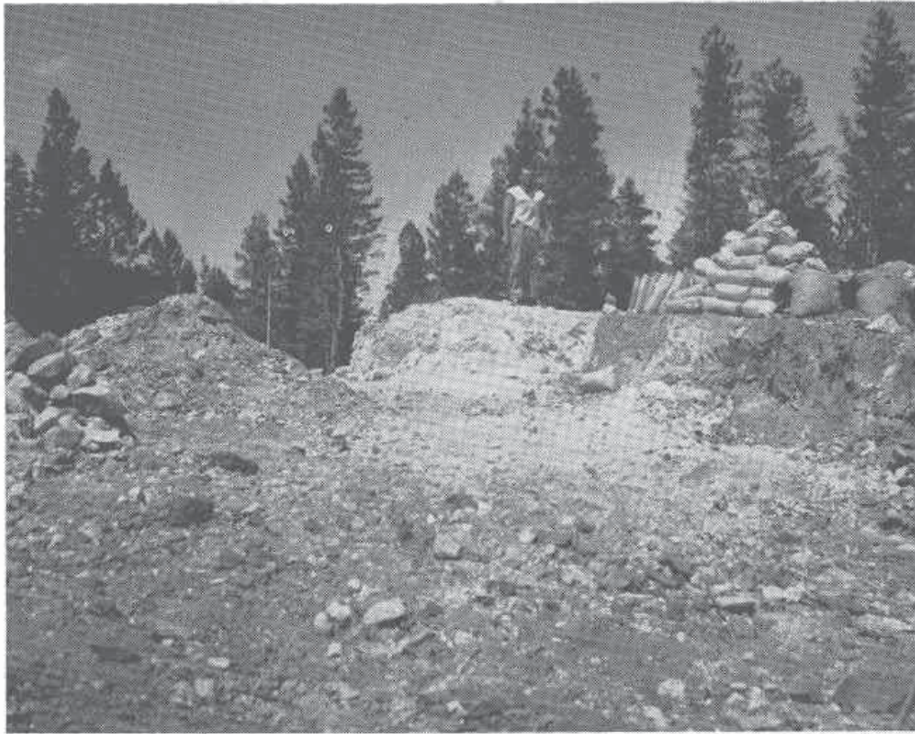
FIG. 2. View of main open cut, Pidlite mine, looking northeast. Note sharp contact between pegmatite and country rock in wall of cut immediately to left of the sacked lepidolite. Man is standing on contact between rib-like mass of quartz (at left) and perthite-quartz-albite pegmatite (at right).
